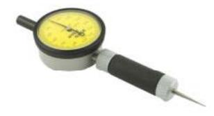
The superior hole gauge is a precision instrument designed to instantly give you a diameter reading in less than two seconds. Merely insert the precision ground, hardened tool steel Gaging Plunger into the hole, press the base of the gage firmly against the part and read the dial directly in 0.001" or 0.02 mm diameter increments on the dial face.
